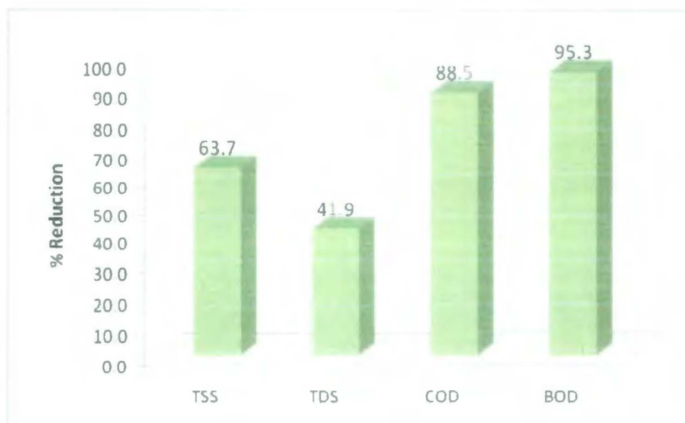
Fig.-5: Performance of Secondary Treatment
